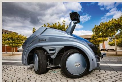
To enable it to perform a wide variety of tasks in even the tightest of spaces in the future, a chassis and drive concept that ensures maximum manoeuvrability was developed for the AI prototype: as a result, the CityBot is capable of driving straight ahead and around bends, as well as diagonally and transversely, and can turn on the spot if necessary. These are functions that no standard road vehicle in the world has yet been able to offer.
